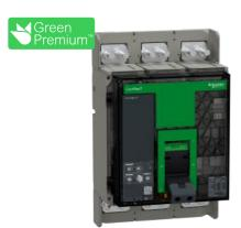
Circuit breaker, ComPacT NS1000N, 50kA at 415VAC, 3P, fixed, manually operated, MicroLogic 2.0 control unit, 1000A
