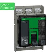
Circuit breaker, ComPacT NS800N, 50kA at 415VAC, 4P, fixed, manually operated, MicroLogic 2.0 control unit, 800A
