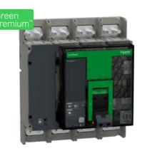
Circuit breaker, ComPacT NS1250H, 70kA at 415VAC, 4P, fixed, manually operated, MicroLogic 2.0 control unit, 1250A
