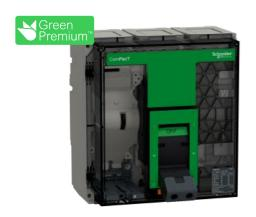
Circuit breaker, ComPacT NS1250H, 70kA at 415VAC, 3P, fixed, manually operated, MicroLogic 2.0 control unit, 1250A
