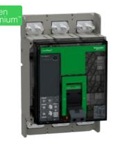
Circuit breaker, ComPacT NS1000N, 50kA at 415VAC, 4P, fixed, manually operated, MicroLogic 2.0 control unit, 1000A
