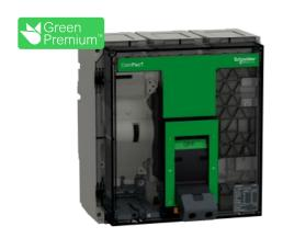
Circuit breaker, ComPacT NS1000H, 70kA at 415VAC, 3P, fixed, manually operated, MicroLogic 2.0 control unit, 1000A
